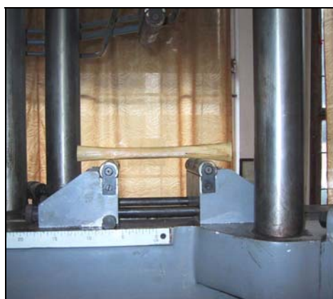
Fig. 5 Testing the bending resistance – probe no. 3
