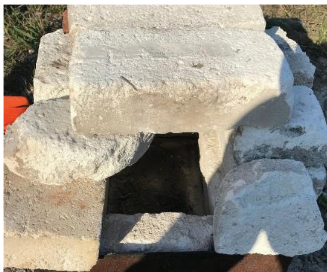
Figure 6. Furnace made out of thermo-insulating bricks, own research.
