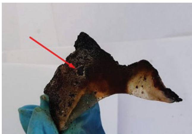
Figure 10. Remainder of complete acrylic prosthesis marked Aerogel-encased NFC. Notice the molten acrylic and the Aerogel acting as a protective film around the NFC tag (own research).
