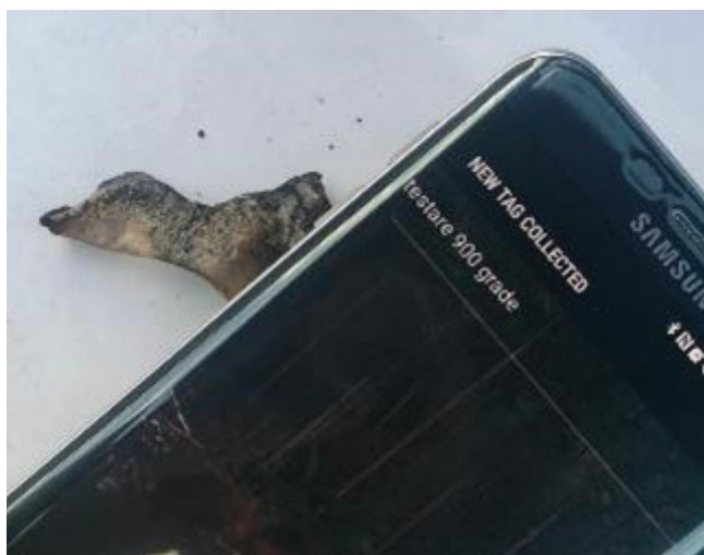
Figure 11. Remainder of prosthesis NFC reading test; the data is readable, signifying that the Aerogel protects the NFC tag at extreme temperature, own research.
