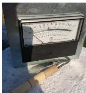
Figure 8. Platinum resistance thermometer placed in the furnace for temperature monitoring, own research.
